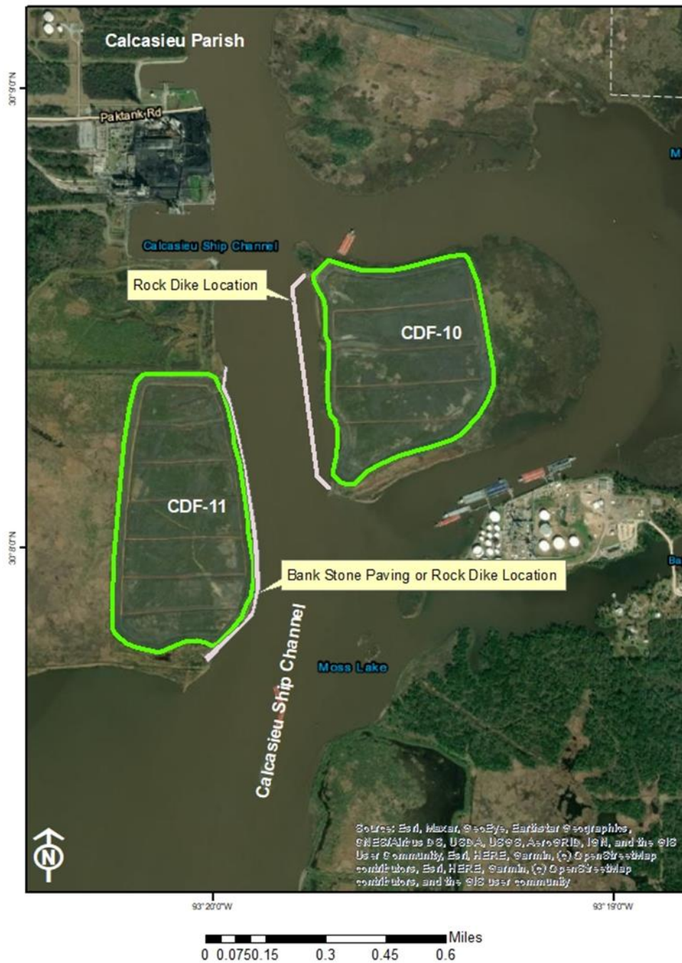
Figure 3. Rock dike location for CDF-10 and bank stone paving or rock dike location for CDF-11
